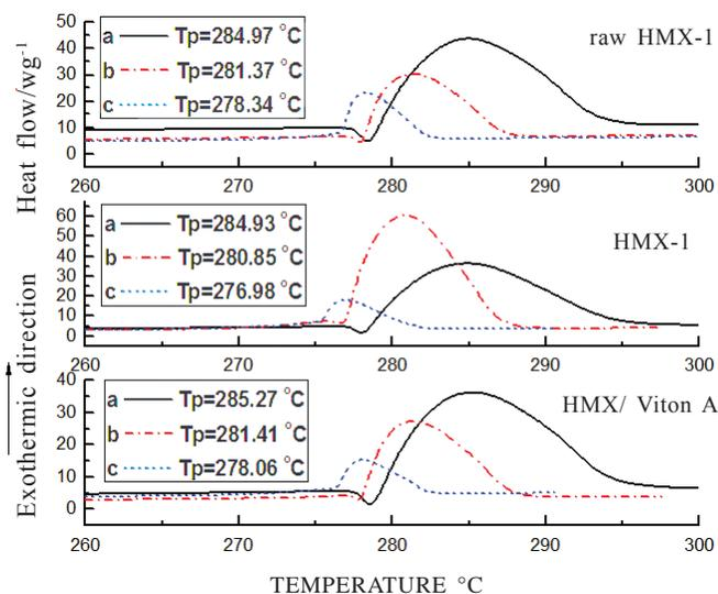
**Figure 4.** DSC curves of raw HMX, HMX-1 and HMX/ Viton A at heating rates of (a) 20 K min<sup>-1</sup>, (b) 10 K min<sup>-1</sup>, and (c) 5 K min<sup>-1</sup>.
