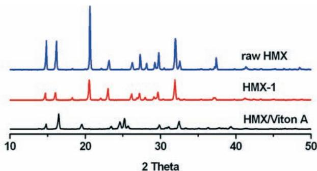
**Figure 3.** X-ray diffraction spectra of raw HMX, HMX-1 and HMX/Viton A nanocomposites.
