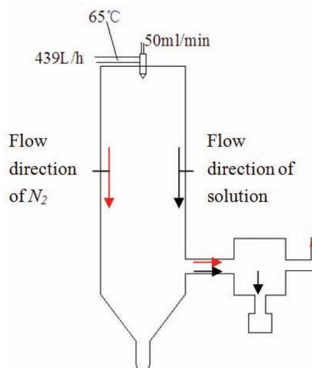
Figure 1. Flow chart of experimental set up.
