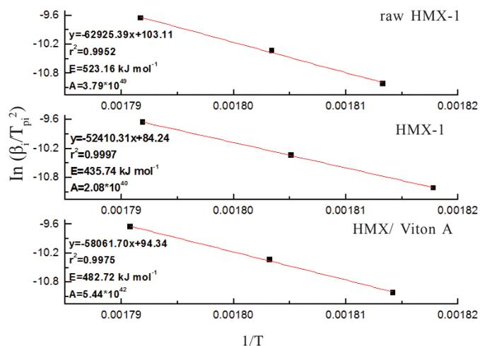
**Figure 5.** Kissinger's plot of raw HMX, HMX-1 and HMX/ Viton A nanocomposites.
