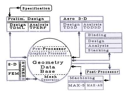
Figure 9. Schematic for integrated design and manufacturing of axial turbines.
