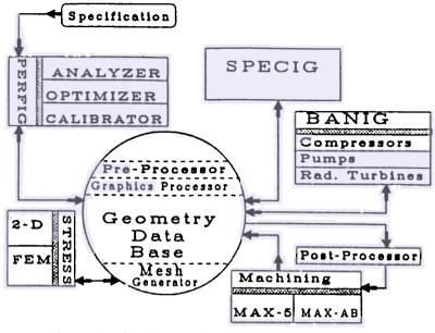
Figure 8. Schematic for integrated design and manufacturing of radial turbomachinery.
