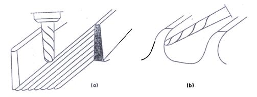
Figure 7. (a) Flank cutting, and (b) point cutting.
