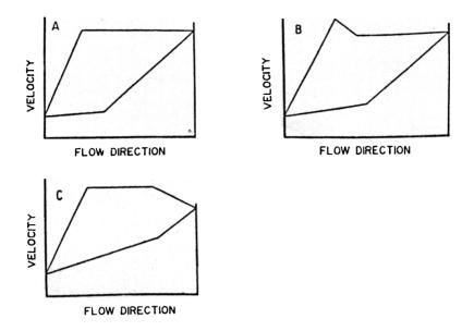
Figure 3. Three types of velocity diagrams in axial turbin
