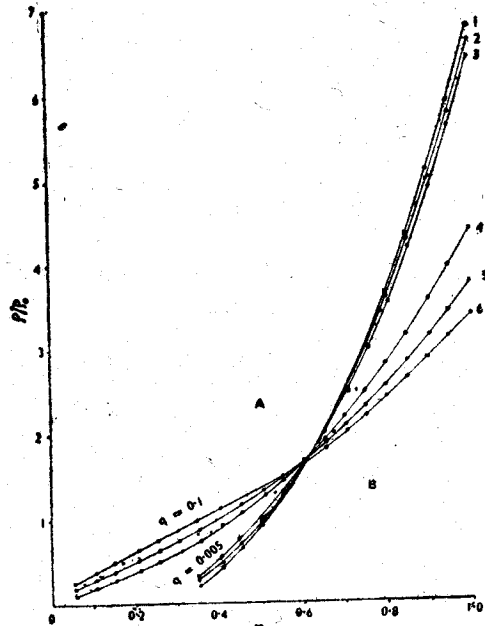
FIG. 2—Density of gas as a function of distance from the centre of symmetry.
