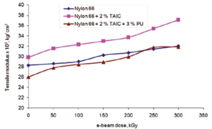
Figure 2. Tensile modulus of various nylon 66 compositions vs dose of e-beam.
