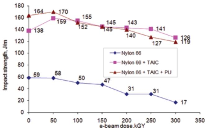
Figure 6. Izod impact strength of various compositions vs dose of e-beam.
