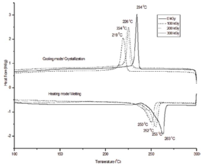
Figure 12. DSC Thermograms for TAIC mixed Nylon 66 at 0, 100, 200 and 300 kGy.
