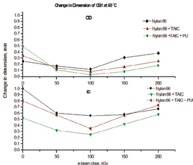
Figure 9. Change in dimension of circular band CB1 at 50 °C with e-beam dose.
