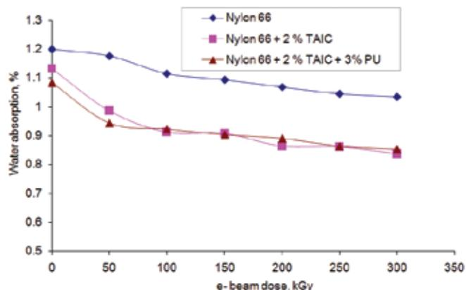
Figure 7. Percent water absorption of various compositions vs dose of e-beam.
