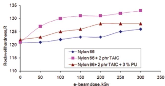
**Figure 5. Rockwell hardness of various compositions vs dose of e-beam.**
