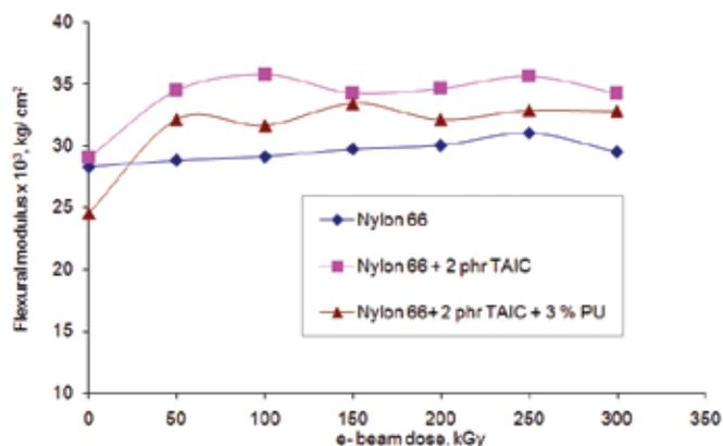
**Figure 4. Flexural modulus of various nylon 66 compositions vs dose of e-beam.**
