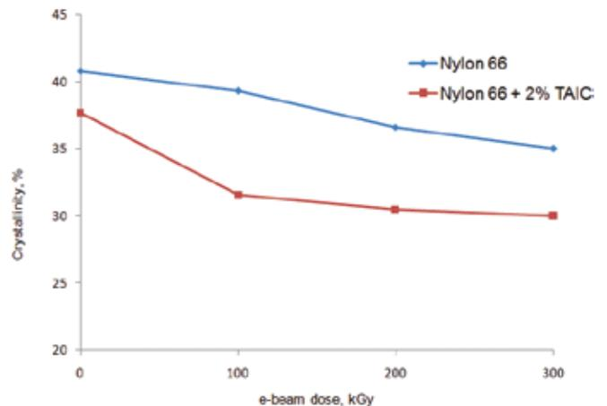
Figure 13. Percent crystallinity of samples as a result of application of different doses of e-beam.
