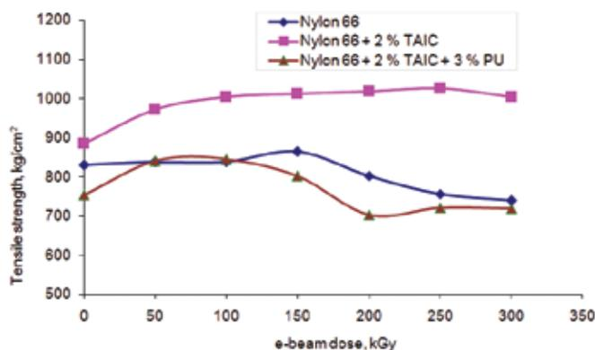
Figure 1. Tensile strength of different nylon 66 compositions vs dose of e-beam.
