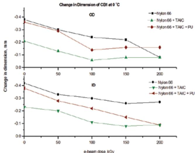
Figure 8. Change in dimension of circular band CB1 at 0 °C with e-beam dose.
