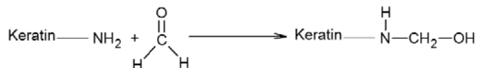
Scheme 3. Formaldehyde absorption by keratin: Available amino groups in keratins chemically interact with formaldehyde
