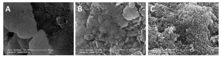
Figure 4. SEM images of Laponite and Laponite containing products (Magnification 250000x): (A) Laponite, (B) Laponite-PAPTMOS, (C) Laponite-PAPTMOS-PANI(MSA).
