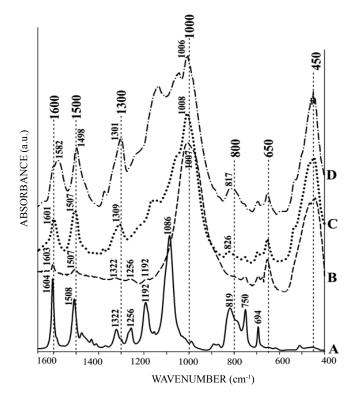
Figure 2. FTIR spectra (mid-wave) of PAPTMOS (A) and the products: (B) Laponite PAPTMOS, (C) Laponite-PAPTMOS-PANI EB, (D) Laponite-PAPTMOS-PANI ES.
