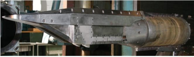
Figure 3. Intake model assembled in the wind tunnel test section.
