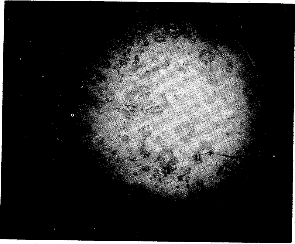
Fig 3.—The dezincification effect. Note the course of dezincification along the contact of the fibre with the surface:
