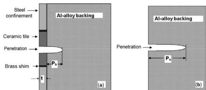
**Figure 1. Schematic of DoP test configuration (a) residual DoP ( $P_b$ ), and (b) reference DoP ( $P_o$ ) in the backing material.**
