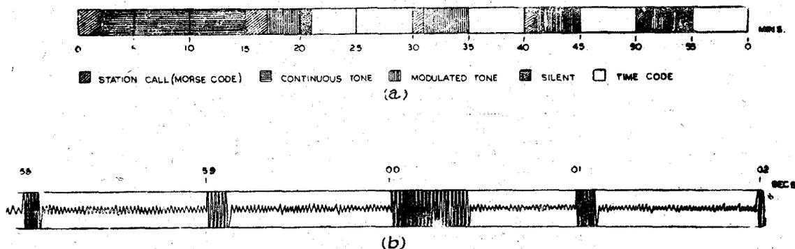
Fig. 1—(a) Hourly broadcast schedule of RWM, Moscow, at 10MHz. The sequence of station call in Morse code, continuous and modulated tones and time code are shown. Time signals are broadcast for 24 minutes every hour
