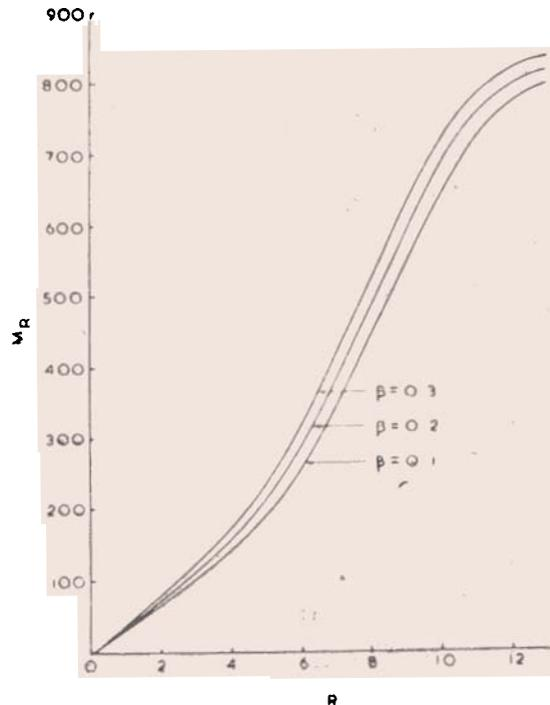
Fig. 3—Variations of the amplitude of oscillations of the heat transfer against dimensionless radius  $R = r (\Omega/\nu)^{\frac{1}{2}}$ .
