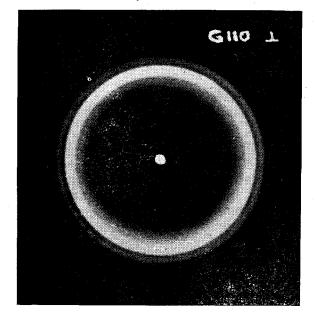
Fig. 2—X-ray diffraction photograph fo polyethylene prepared at  $110^{\circ}$ C between glass plates. X-rays perpendicular to thickness (distance r=4 cm).
