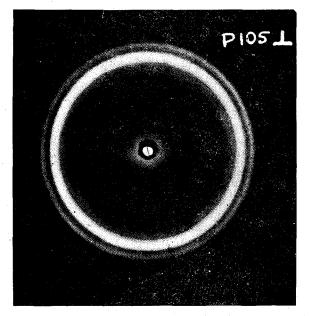
Fig. 3-X-ray diffraction photograph of polyethylene sample prepared at 105°C between perspex plates. X-rays perpendicular to thickness (distance r=6 cm).
