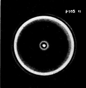
Fig. 5—X-ray diffraction photograph of polyethylene prepared at 110 °C between glass plates. X-rays parallel to thickness (distance r=4 cm).
