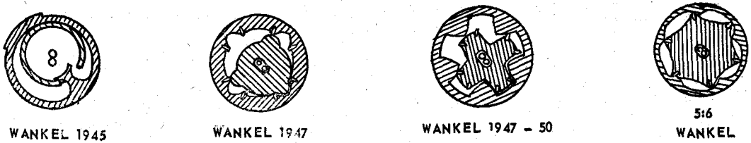
Fig. 4—Various configurations of Wankel Engine.
