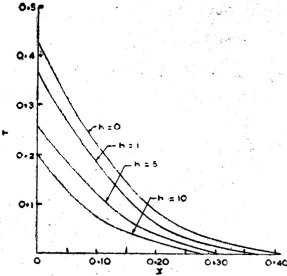
Fig 1—Temperature distribution at various time in the slab at  $v=1/3$ .
