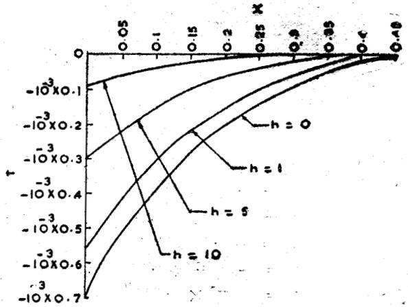
Fig 2—Temperature distribution at various time in the slab at  $v=1/2$ .
