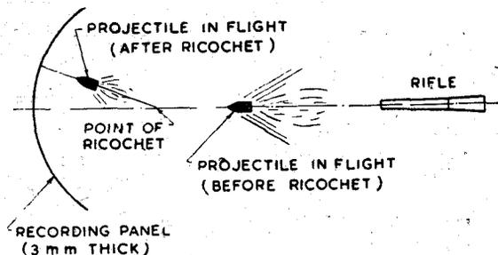
Fig. 2—Experimental set-up for determining different ricochet parameters.
