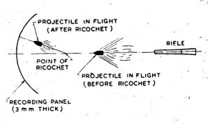
Fig. 2—Experimental set-up for determining different ricochet parameters.
