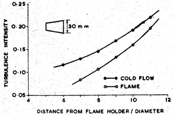
Fig. 4—Turbulence intensity behind a truncated cone.
