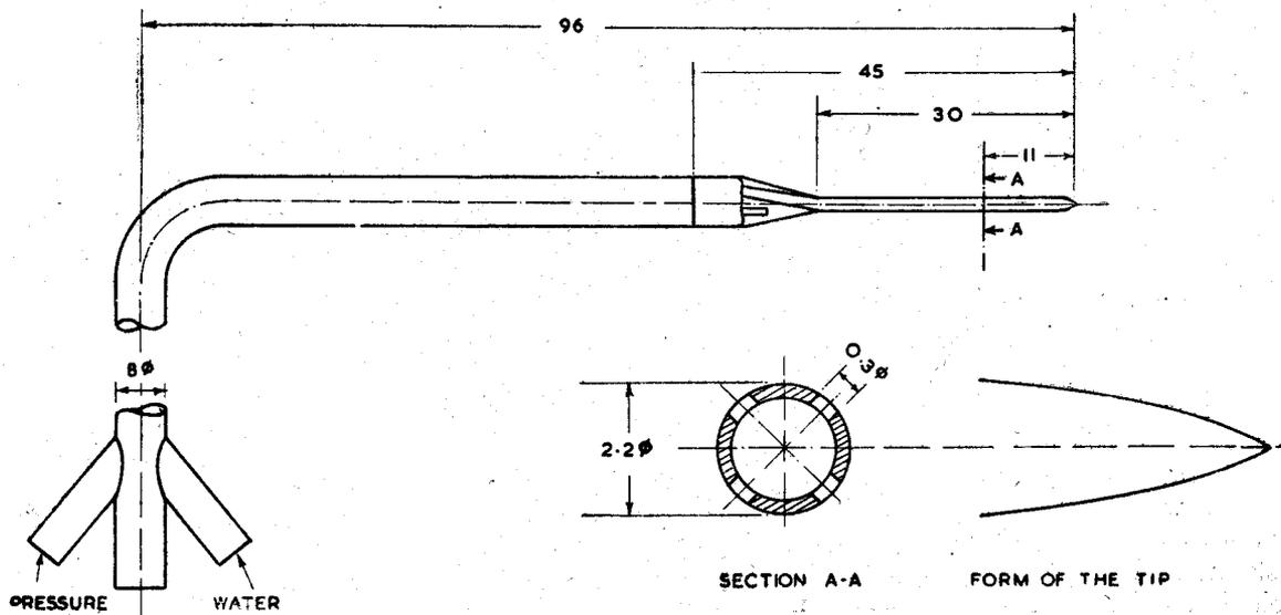
Fig. 1—Static pressure probe.
