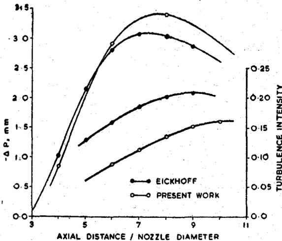
Fig. 2—Variation in static pressure defect and turbulence intensity in a free jet.
