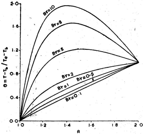
Fig. 3—Response of temperature in pseudoplastic fluid ( $n = 1/3$ ) to an increase in Brinkman number  $Br$  at fixed Peclet number  $Pe' = 10$  in a rotating annulus.
