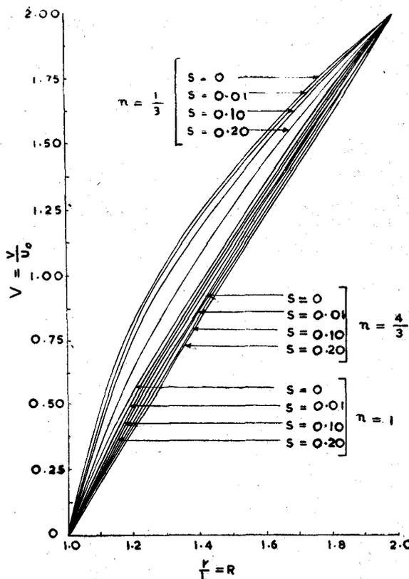
which shows that whether the walls are solid or porous, even the first order solution exhibits the effect of Power-Law index  $n$  on the flow pattern. Putting  $n=1$  in (57) we obtain the results obtained by Bird *et al*<sup>3</sup>.
