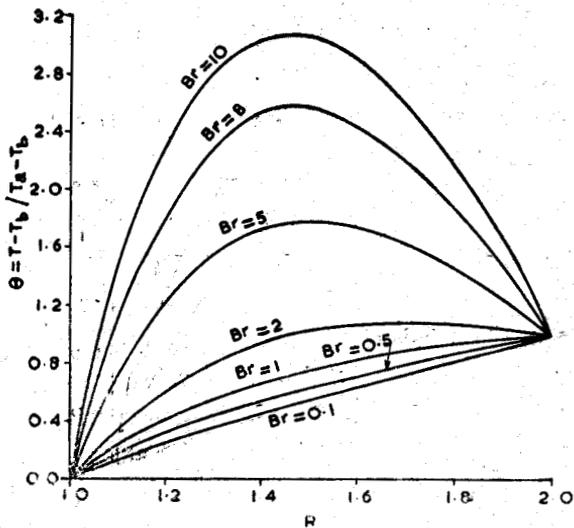
Fig. 7—Variation of temperature in dilatant fluid ( $n = 4/3$ ) with Brinkman number ( $Br$ ) at fixed  $Pe' = 10$ .
