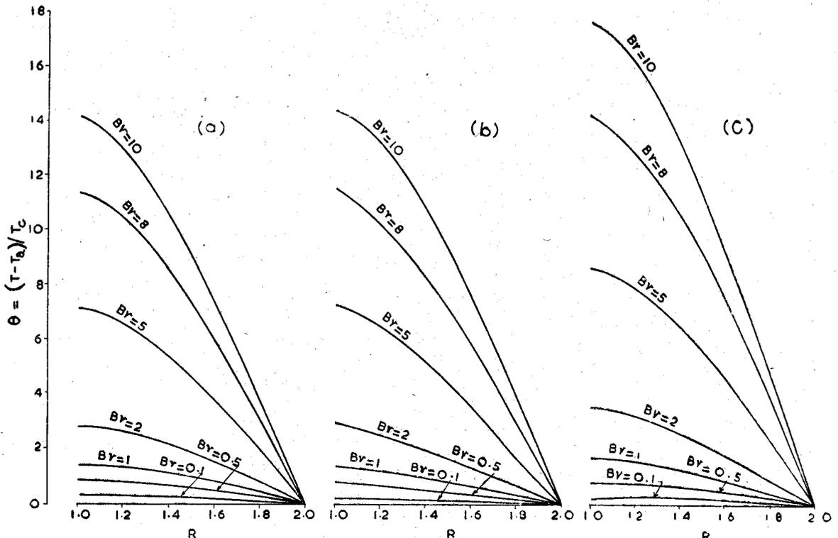
Fig. 9 (a, b, c)—Temperature distribution in power-law fluids in a rotating cylindrical annulus (inner wall insulated) for various Brinkman numbers ( $Br$ ). Where for : (a)  $n=1/3, Pe'=10, S=0.1$ . (b)  $n=1, Pe'=10, S=0.1$ . (c)  $n=4/3, Pe'=10, S=0.1$ .
