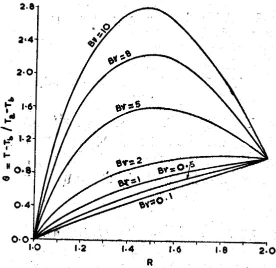
Fig. 5—Response of temperature in Newtonian fluids ( $n = 1$ ) in a rotating annulus to an increase in Brinkman number ( $Br$ ) at fixed  $Pe' = 10$ .
