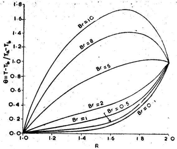
Fig. 6—Response of temperature in Newtonian fluid ( $n = 1$ ) to increase in Brinkman number ( $Br$ ) at  $Pe' = 100$  in rotating annulus.
