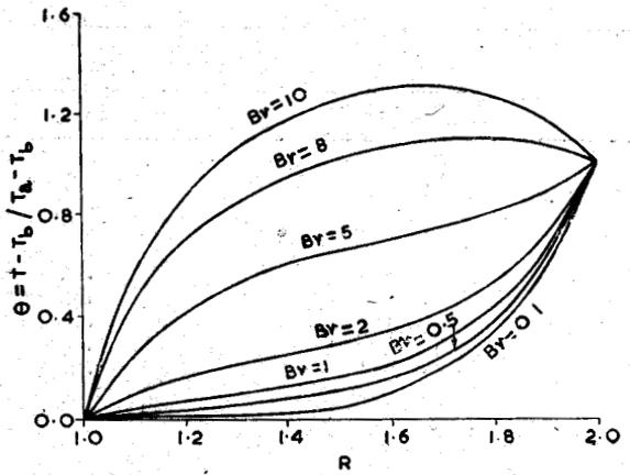
Fig. 4—Response of temperature in pseudoplastic fluid ( $n = 1/3$ ) to increase in Brinkman number ( $Br$ ) at fixed  $Pe' = 100$  in a rotating annulus.
