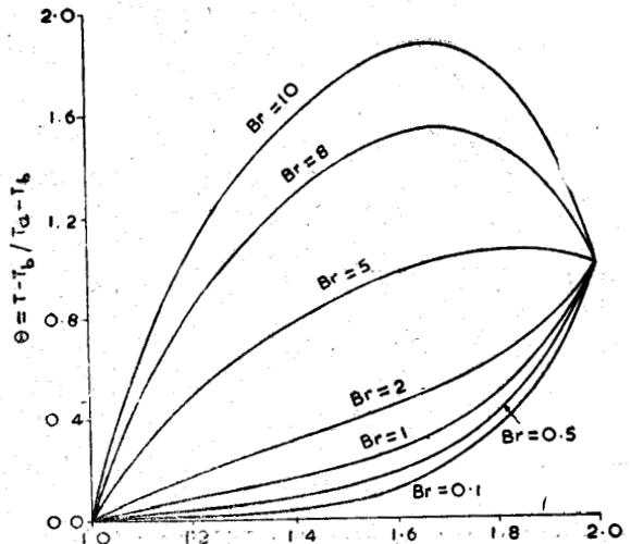
Fig. 8—Variation of temperature in dilatant fluid ( $n = 4/3$ ) with Brinkman number ( $Br$ ) at fixed  $Pe' = 100$ .
