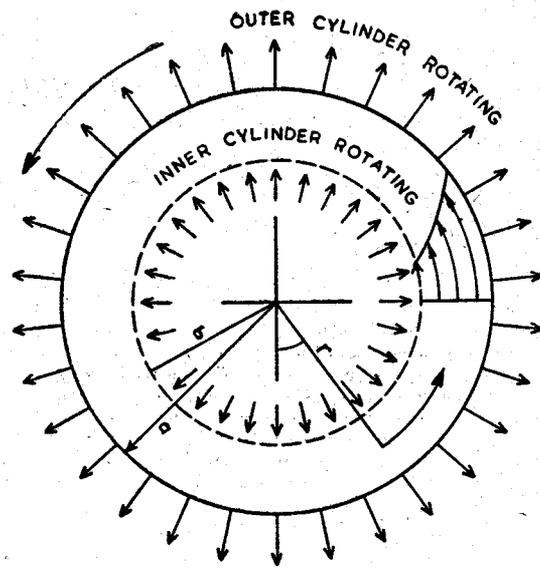
Fig. 1—Tangential flow of power-law fluids in an annulus between two rotating co-axial cylinders.
