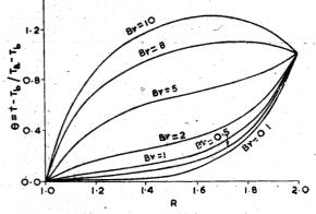
Fig. 4—Response of temperature in pseudoplastic fluid (n = 1/3) to increase in Brinkman number (Br) at fixed Pe' = 100 in a rotating annulus.
