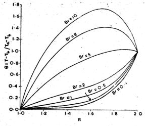
Fig. 6—Response of temperature in Newtonion fluid (n = 1) to increase in Brinkman number (Br) at Pe' = 100 in rotating annulus.
