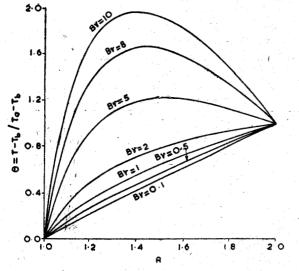
Fig. 3—Response of temperature in pseudoplastic fluid (n = 1/3) to an increase in Brinkman number Br at fixed Peelet number Pe' = 10 in a rotating annulus.
