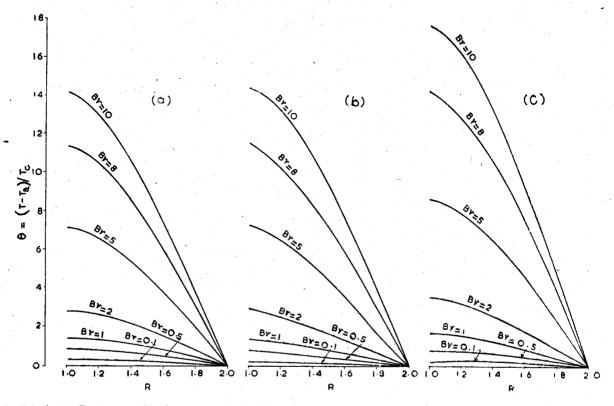
Fig. 9 (a, b, c)—Temperature distribution in power-law fluids in a rotating cylinderical annulus (inner wall insulated) for various Brinkman numbers (Br.) Where for : (a) n=1/3, Pe'=10,  $S=0\cdot1$ . (b) n=1, Pe'=10,  $S=0\cdot1$ . (c) n=4/3. Pe'=10,  $S=0\cdot1$ .
