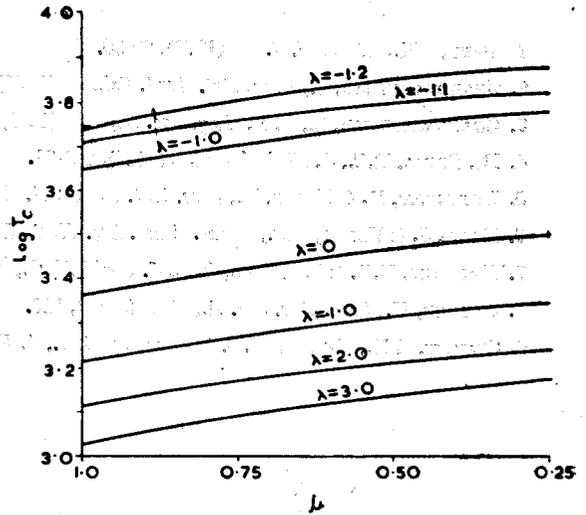
Fig. 3—The variation of the log of the critical Taylor number  $T_c$  with  $\mu$  for  $R=20.0$ ,  $\sigma = -55.70$  and  $\alpha = 3.40$ . The values of  $\lambda$  are shown on the curves.
