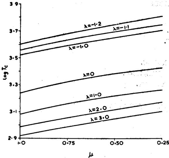
Fig. 2—The variation of the log of the critical Taylor number  $T_c$  with  $\mu$  for  $R=5.0$ ,  $\sigma = -12.6$  and  $\alpha = 3.1$ . The values of  $\lambda$  are shown on the curves.
