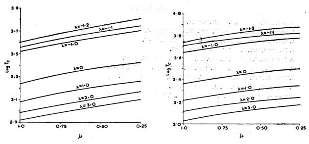
Fig. 2—The variation of the log of the critical Taylor number Tc with  $\mu$  for R=5.0,  $\sigma=-12.6$  and a=3.1. The values of  $\lambda$  are shown on the curves.
