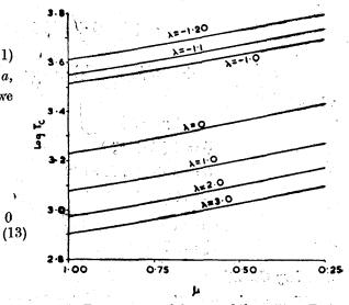
Fig. 1—The variation of the log of the critical Taylor number  $T_{0}$  with  $\mu$  for R=0,  $\sigma=0$  and a=3.12. The values of  $\lambda$  are shown on the curves.
