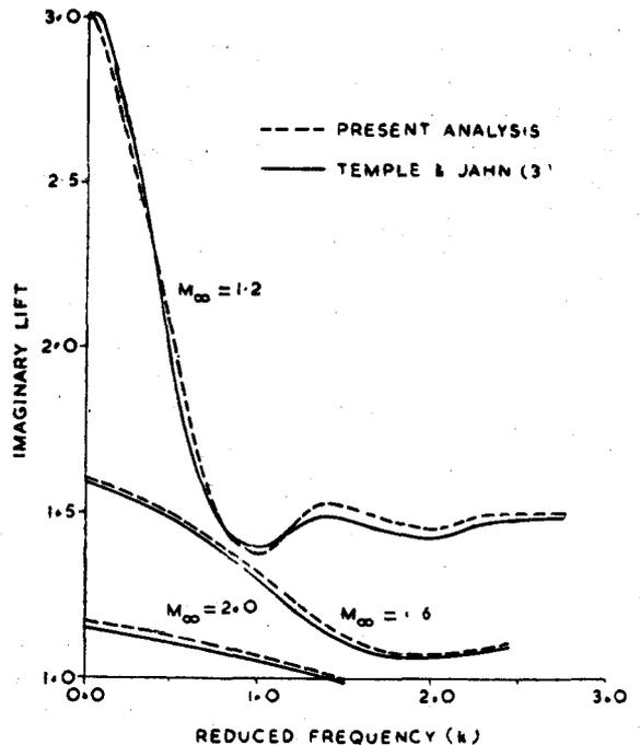
Fig. 2—Values of the imaginary part of the lift against  $k$  for  $M_\infty = 1.2, 1.6 \text{ and } 2.0$ .
