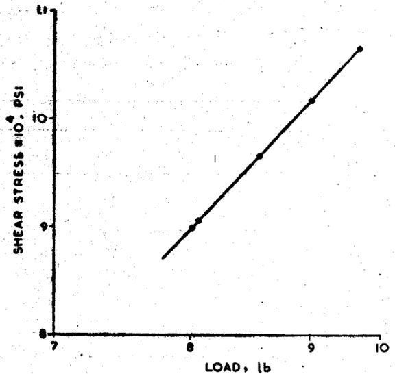
Fig. 7—Variation of shear stress with load at -40° C
