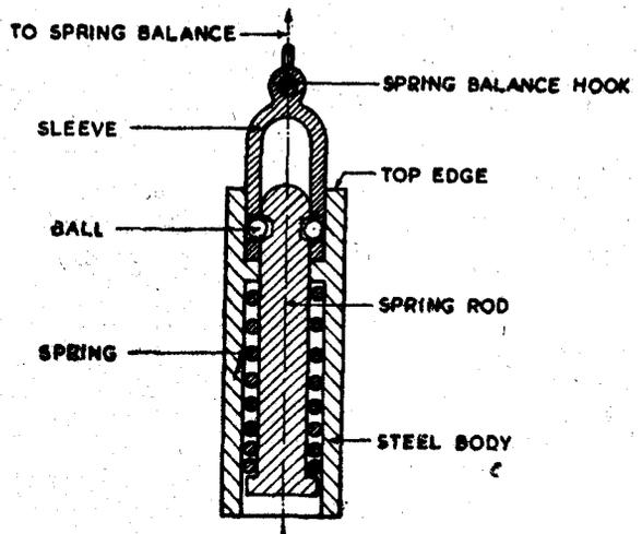
Fig. 1—Test set-up.
