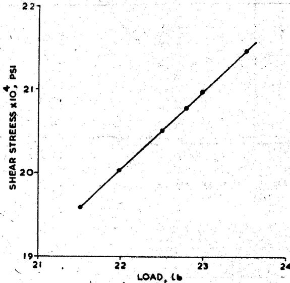
Fig. 2—Variation of shear stress with load at 20°C
