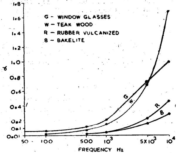
FIG. 4—Variation of attenuation constant ( $\alpha$ ) with frequency.
