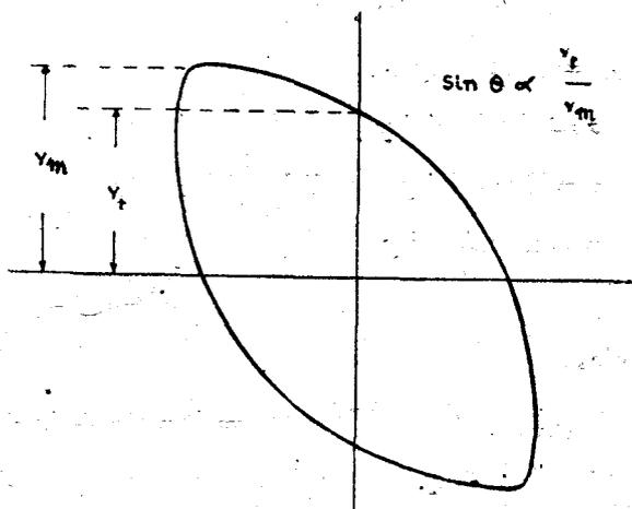
FIG. 2—Ellipses at different working points (frequency) as seen on C.R.O,
