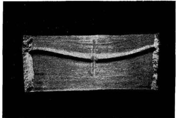
Fig. 8—Impression of the groove on the driving band after pressing and the lines of flow of the material into the undercut.
