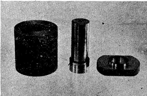
Fig. 1—Die set used for compacting 40 mm I.D. annular rings.
