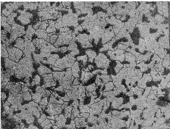
Fig. 5—Pure ferrite grains with inter-connected Porosity after sintering Fe A at 1150°C for 4 hours (X 200) etchant : 1.5% nital solution.
