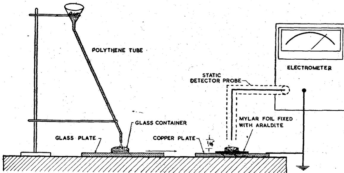
Fig. 1—Experimental set-up for static charge measurement.
