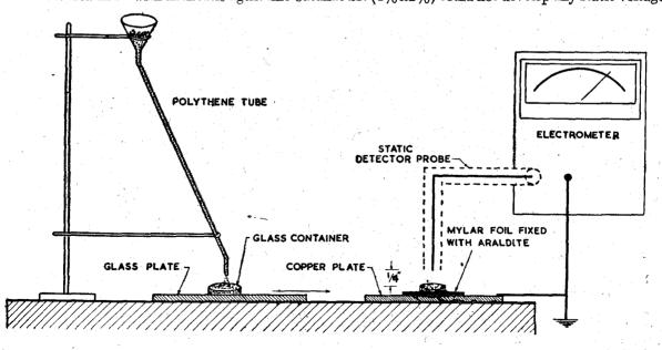
Fig. 1-Experimental set-up for static charge measurement.
