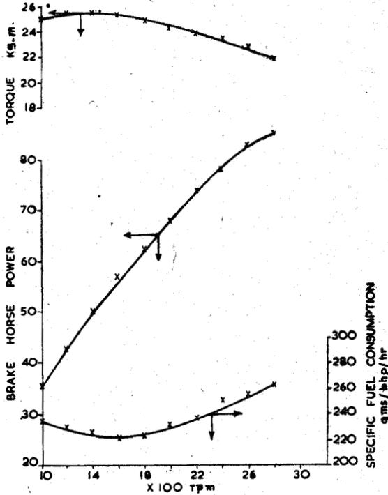
Fig. 2—Performance of an automotive diesel engine at ambient conditions.
