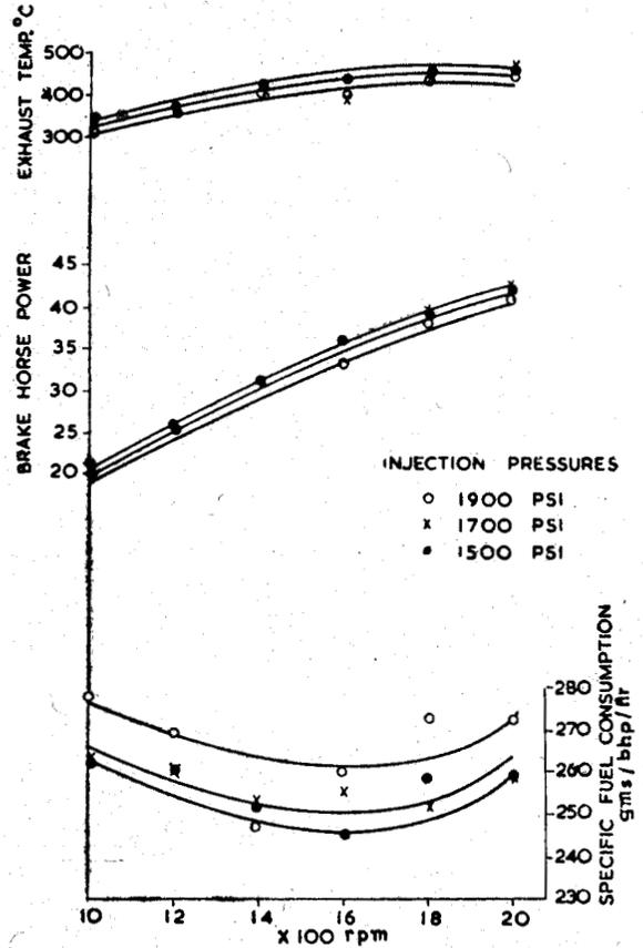
Fig. 3—Performance at simulated altitude conditions corresponding to 2600 m, varying the injection pressures.
