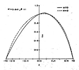
Fig. 1-Normalized velocity rofiles of the primary flow,
