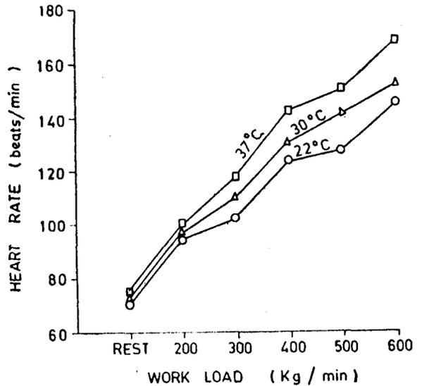
Fig. 1—Changes in heart rate against graded work at three ambient temperatures.
