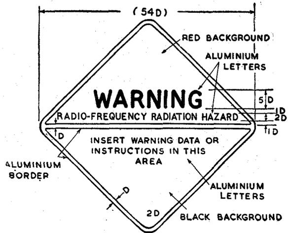
Fig. 8—Radio-frequency radiation hazard warning symbol.
