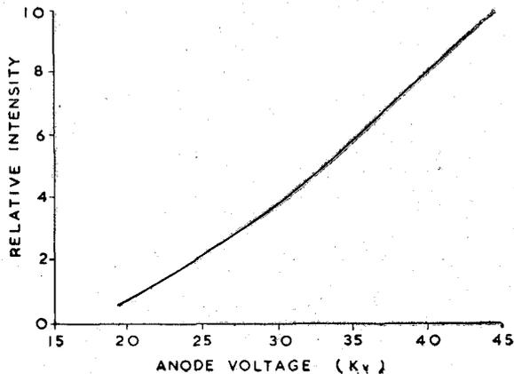
Fig. 7—Relative intensity of X-rays as a function of anode voltage.
