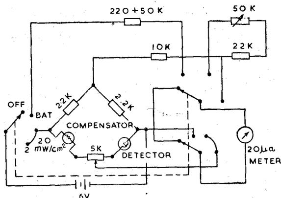
Fig. 1—Microwave radiation monitor (circuit).
