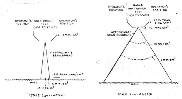
Fig. 5—High power radiation test-lock on mode.
