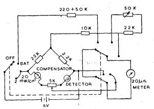
Fig. 1-Microwave radiation monitor (circuit).
