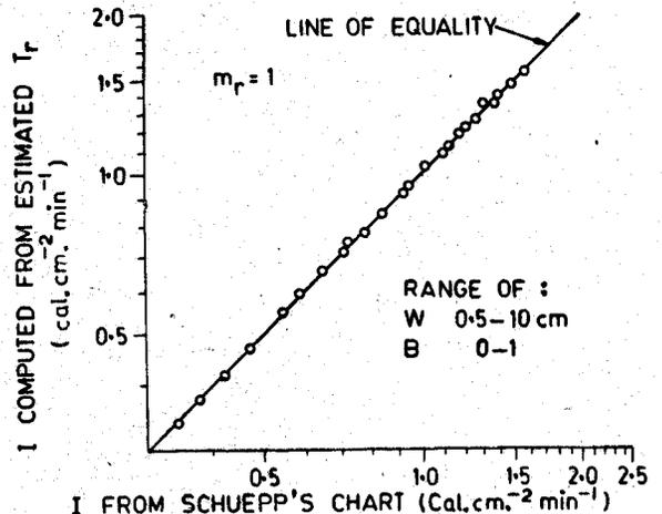
Fig. 4  $I$  computed from proposed formula compared with  $I$  obtained from schuepp's chart for different values of 'W' & 'B' at unit air mass.
