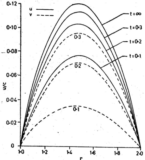
Fig. 4—Velocity profile of fluid and particles for values of  $t$  indicated when  $f = 0.1$ ,  $\tau = 0.1$  and  $M = 1$ .
