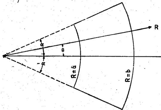
Fig. 2—Geometry of cross section (Case 4) and coordinate system.
