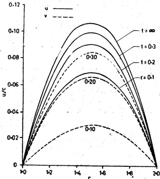
Fig. 5—Velocity profile of fluid and particles for values of  $t$  indicated when  $f = 0.1$ ,  $\tau = 0.1$  and  $M = 2$ .
