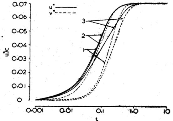
Fig. 7—Mean velocity of the fluid and particles for (1)  $f = 0.10$ ,  $\tau = 0.10$ ; (2)  $f = 0.10$ ,  $\tau = 0.01$  and (3)  $f = 1.0$ ,  $\tau = 0.10$  and  $M = 2$ .
