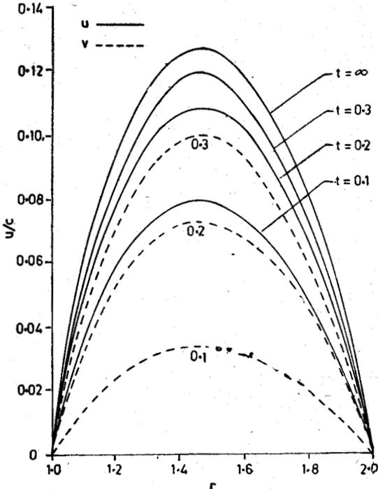
Fig. 3—Velocity profile of fluid and particles for values of  $t$  indicated when  $f = 0.1$ ,  $\tau = 0.1$  and  $M = 0$
