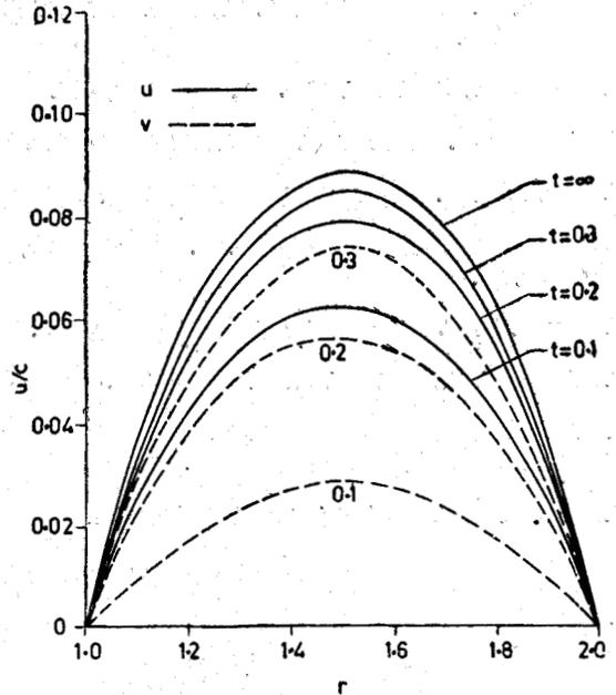
Fig. 6—Velocity profile of fluid and particles for values of  $t$  indicated when  $f = 0.1$ ,  $\tau = 0.1$  and  $M = 3$ .
