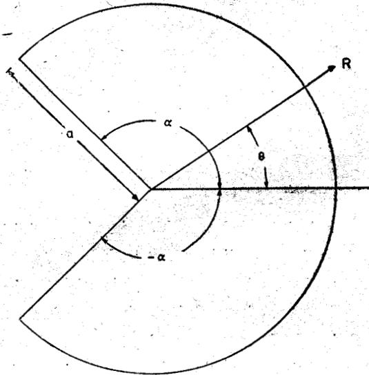
Fig. 1—Geometry of cross-section and coordinate system (Case 3).
