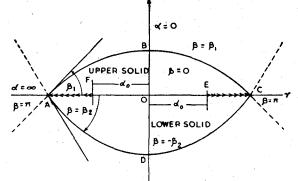
The temperature distributions in two plano-convex solids ABCOA & ADCOA is here considered. The total region ABCDA is formed by two intersecting spheres as shown in the Fig. 1. EC and FA portions of the cemented surfaces of the solids are perfectly invalated and A and C are rigidly connected. In the upper solid the temperature function is prescribed along ABC. Hence we have the boundary conditions:
