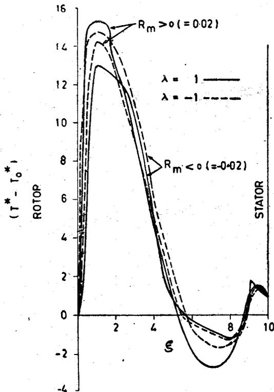
Fig. 5—Variation of  $(T^* - T_0^*)$  for no-recirculation for  $Rz = 40$ ,  $x = 1.0$ .
