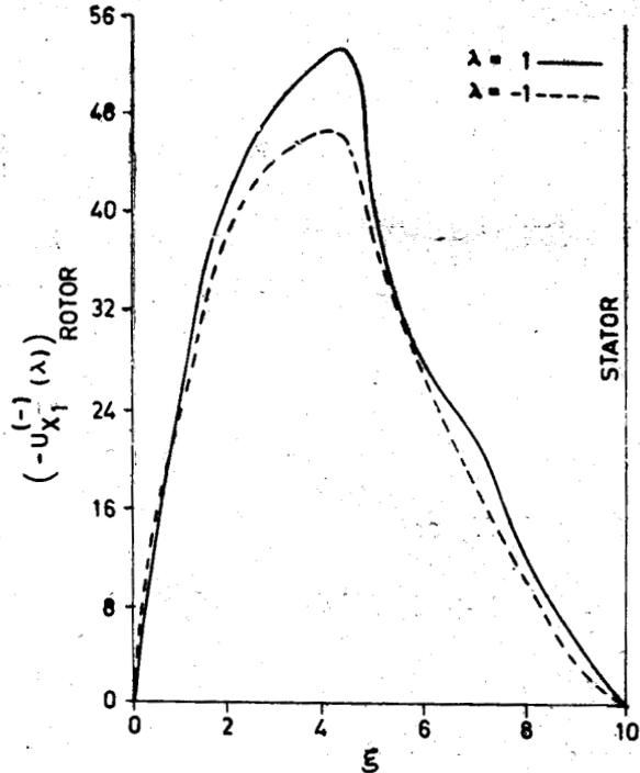
Fig. 1—Variation of radial velocity for maximum radii for no-recirculation (for  $Rm > 0$ ).
