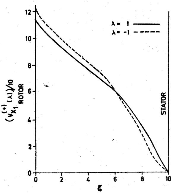
Fig. 3—Variation of transverse velocity for maximum radii (for  $R_m > 0$ ) for no-recirculation.
