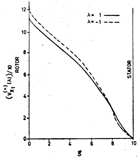
Fig. 4—Variation of transverse velocity for maximum radii (for  $R_m < 0$ ) for no-recirculation.
