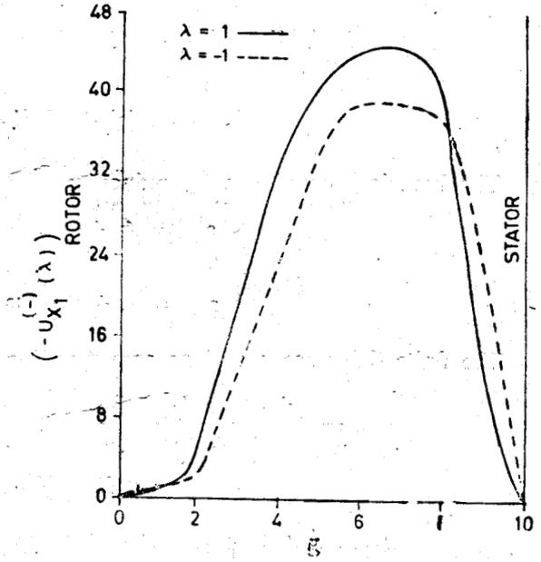
Fig. 2—Variation of radial velocity for maximum radii (for  $Rm < 0$ ) for no-recirculation.
