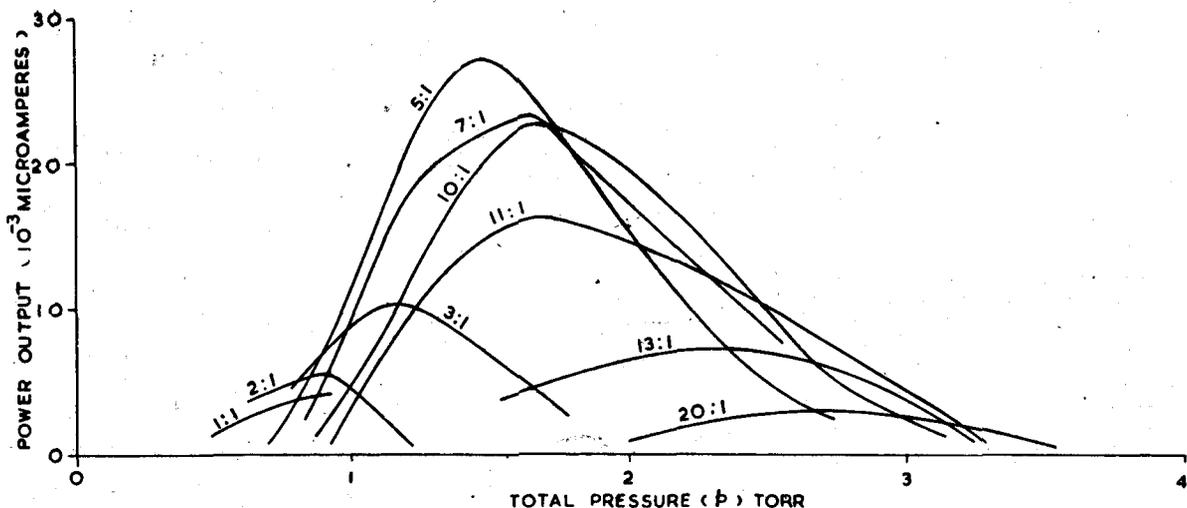
Fig. 4—Variation of laser power output vs total pressure for different mixture ratios in He-Ne gas laser (6328A°).
