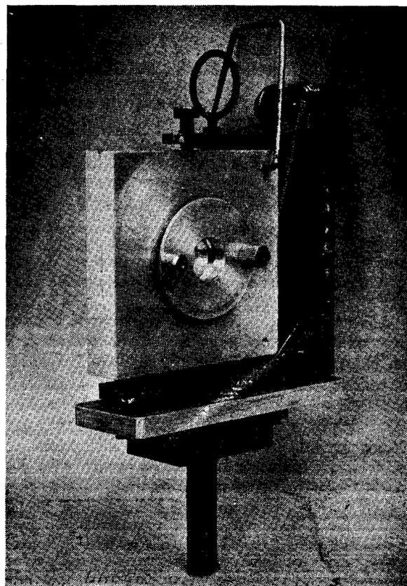
Fig. 2—Laser mirror mounts. These were specially fabricated to have spring loaded screws for finer adjustment of the tilt of the mirror.
