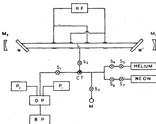
Fig. 1—Experimental set-up for *He-Ne* gas laser. ( $S_1, \dots, S_7$ )=High vacuum stop cocks; CT=Cold trap of liquid  $N_2$ ; M=Oil manometer; L=Laser tube; W=Brewster windows of fused quartz;  $M_1, M_2$ =Multilayer dielectric coated mirrors; RF=Radio frequency oscillator; DP=Oil diffusion pump; BP=Backing pump;  $P_1$ =Pirani gauge;  $P_2$ =Penning gauge.
