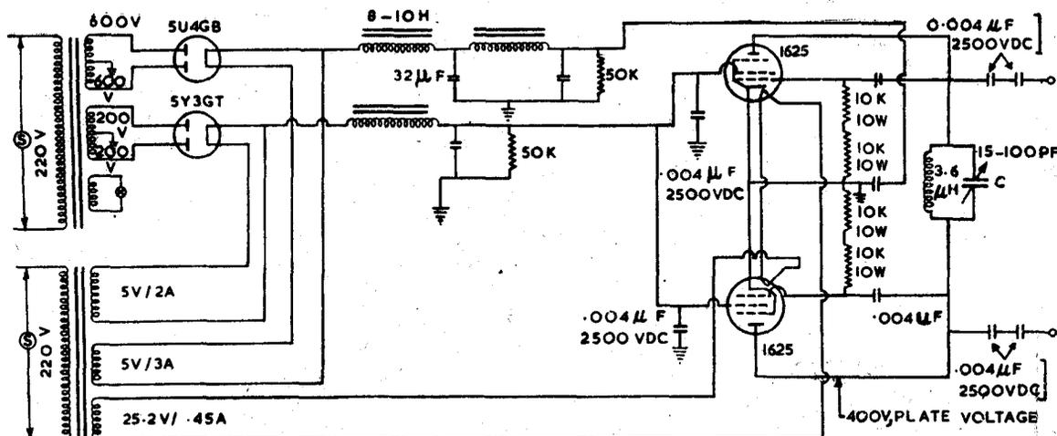
Fig. 3—Radio Frequency Oscillator.
