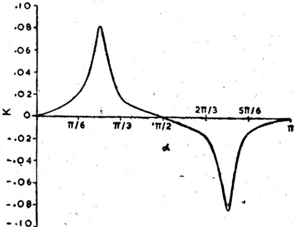
The value of  $K$  remains constant for a particular plate but varies as  $\alpha$ , the angle between the elastic axes of the material and the physical boundary line, takes different values. For an Oak plate with  $p_1 = 5/3$ ,  $p_2 = 49/51$ , the value of  $K$  for different values of  $\alpha$  has been given below and graphically represented in Fig. 2.
