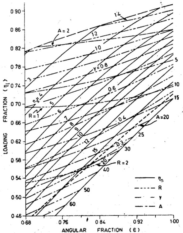
Fig. 3—Design graph for single propellant star grain with parametric values of  $y, \eta_s, A$  and  $R$ ;  $n=7, f=0.12$  and  $\theta=0.9$ .
