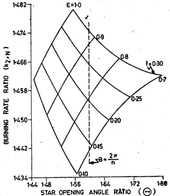
Fig. 8—Conditions of neutral burning for the four pointed dual propellant grain;  $\nu=0$  and  $n=4$ .
