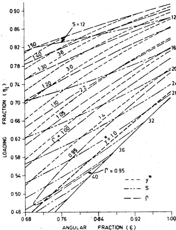
Fig. 2—Design graph for single propellant star grain with parametric values of  $y^*$ ,  $S$  and  $\Gamma$ ;  $n=7, f=0.12$  and  $\theta=0.9$ .
