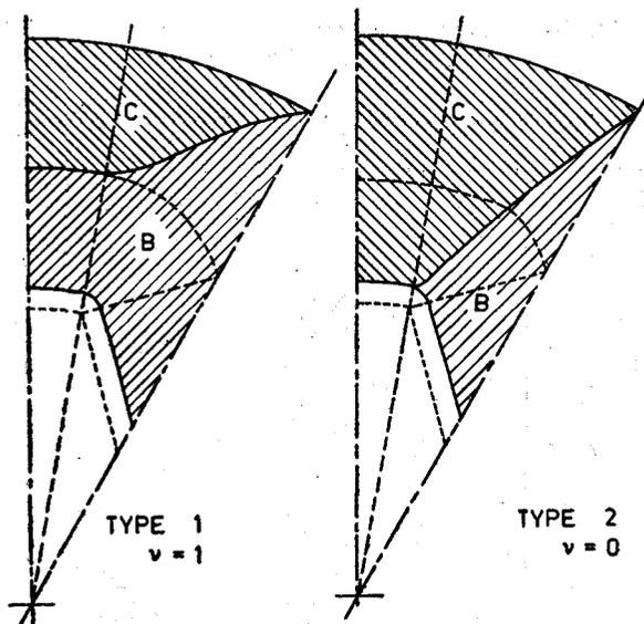
Fig. 4—Dual propellant grains.
