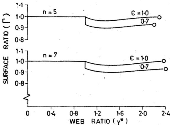
Fig. 7—Comparison of surface ratio variation of near neutral burning dual propellant grains;  $\nu=1$  and  $f=0.1$ .
