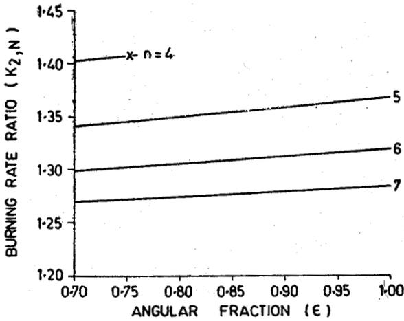
Fig. 5—Burning rate ratio requirement for near neutral burning dual propellant grains;  $\nu=1$  &  $f=0.1$ .
