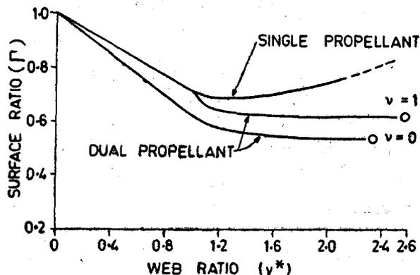
Fig. 10—Booster-sustainer combination in dual propellant grains;  $n=8$ ,  $\theta=\pi/4$ ,  $\epsilon=1$ ,  $f=0.1$  and  $k_2=1.3$ .
