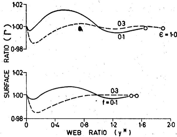
Fig. 9—Comparison of surface ratio variation of near neutral burning dual propellant grains;  $\nu = 0$  and  $n = 5$ .
