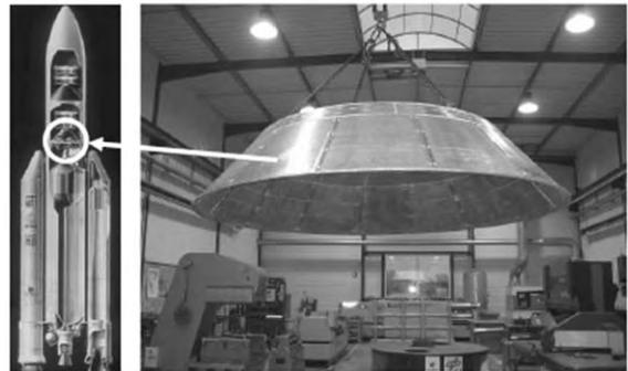
**Figure 8. Ariane 65 rocket cone prototype made of aluminium foam sandwich. Arrow shows the location of part in the rocket<sup>21</sup>.**
