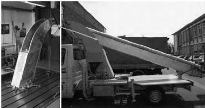
**Figure 6. Base of a lifting arm made from aluminium foam sandwich panels<sup>19</sup>.**
