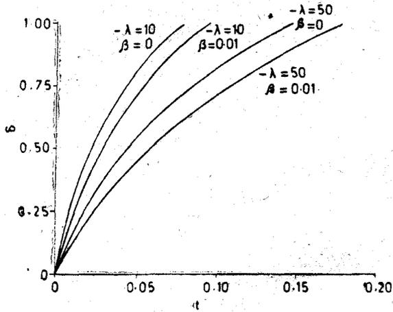
Fig. 3—Boundary layer thickness against time (4th degree profile).
