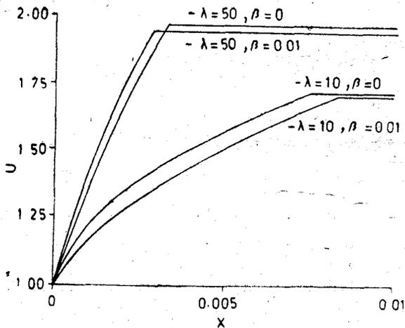
Fig. 5—Core velocity against axial distance (4th degree profile).
