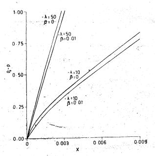
Fig. 6—Pressure drop against axial distance (4th degree profile).
