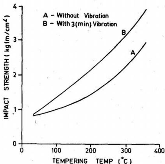
Figure 15. Tempering temperature vs impact strength, 0.5% carbon steel.
