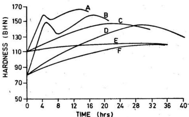
Figure 3. Ageing curve, Material 7075. A—140°C with US, B—140°C without US, C—80°C with US, D—80°C without US, E—RT (30°C) with US, F—RT (30°C) without US.
