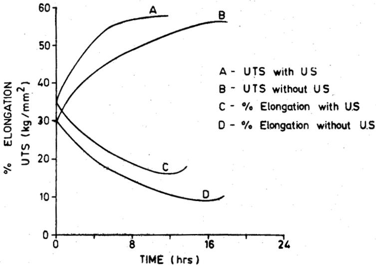
Figure 12. UTS and percentage elongation vs time, material 7075.
