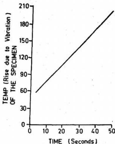
Figure 16. Vibration time vs temp of specimen (°C) without cooling.
