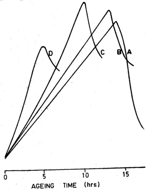
Figure 7. Ageing time vs hardness (varying vibration period), duralumin 2024 aged at 170°C. A—0 min per hour of ageing, B—1 min per hour of ageing, C—2 min per hour of ageing, D—5 min per hour of ageing.
