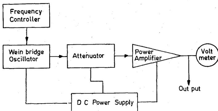
Figure 1. Variable frequency power supply unit.
