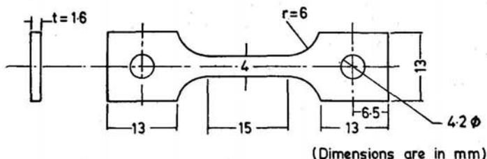
Figure 2. Tensometer Specimen.
