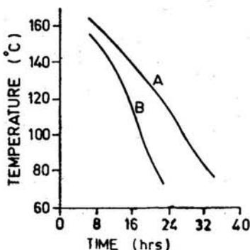
Figure 4. Temperature vs time to reach maximum hardness, material 7075. A—without US. B—with US.
