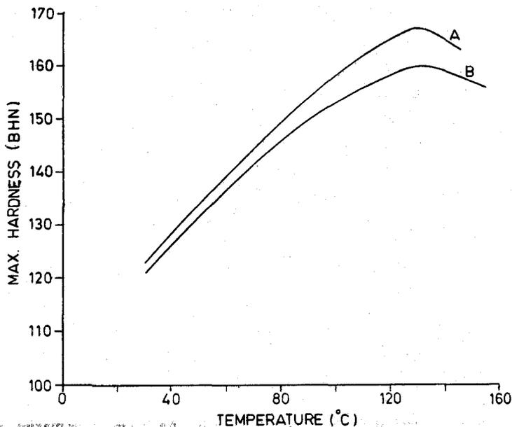
Figure 5. Maximum hardness vs temperature, material 7075. A— with US, B— without US.
