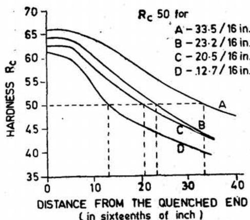
Figure 13. Hardenability curve, high carbon steel (1% C). A—water quenched with US, B—water quenched without US, C—oil quenched with US, D—oil quenched without US.
