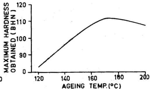
Figure 9. Ageing temp. vs maximum hardness.
