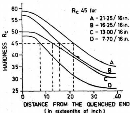
Figure 14. Hardenability curve, material 4140. A—water quenched with US, B—water quenched without US, C—oil quenched with US, D—oil quenched without US.
