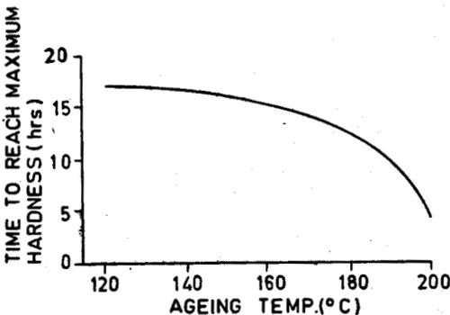
Figure 8. Ageing temp. vs time to reach maximum hardness, duralumin 2024.
