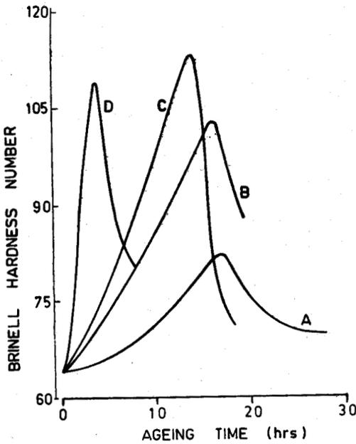
Figure 6. Ageing time vs hardness (without vibration), duralumin 2024. A—aged at 120°C, B—aged at 150°C, C—aged at 170°C, D—aged at 200°C.
