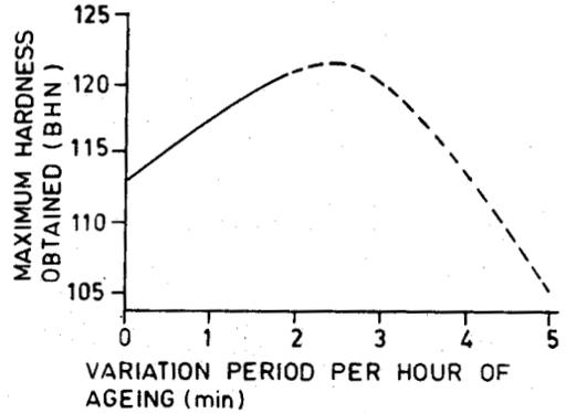
Figure 11. Ageing temp. vs maximum hardness, duralumin 2024, aged at 170°C.
