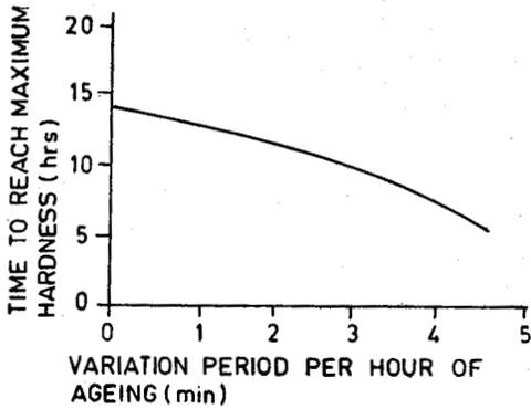
Figure 10. Vibration period vs time to reach maximum hardness, duralumin 2024 aged at 170°C.
