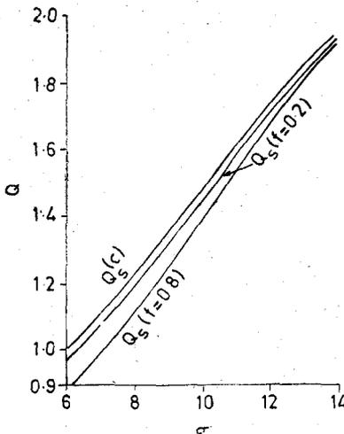
**Figure 1.** Graph shows flux  $Q$  against  $\sigma$ , where  $Q_s^{(c)}$  = clean fluid flux and  $Q_s$  = dusty fluid flux.
