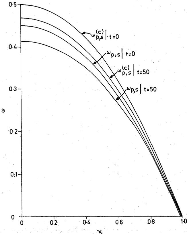
Figure 2. Velocities of clean and dusty fluids flowing between parallel plates.
