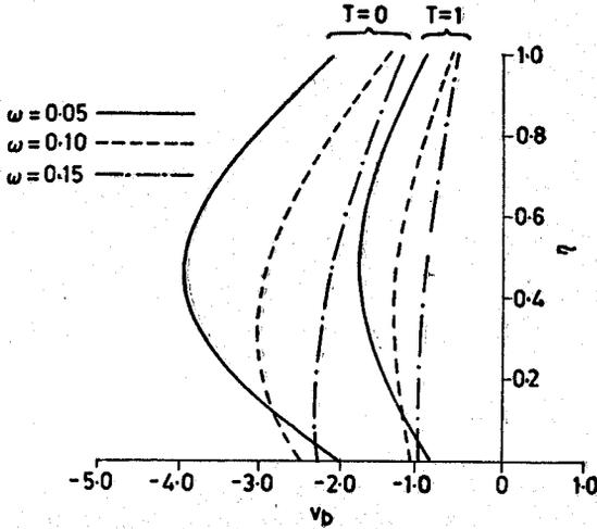
Figure 4. Velocity distributions of the dust particle in a direction normal to the direction of motion of the plate.
