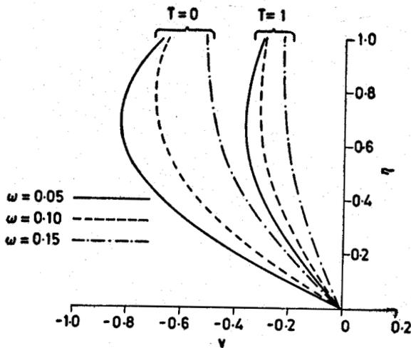
Figure 2. Velocity distributions of the dusty gas in a direction normal to the direction of motion of the plate.
