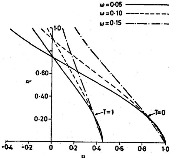
Figure 1. Velocity distributions of the dusty gas along with the direction of motion of the plate.
