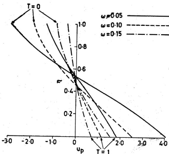
Figure 3. Velocity distributions of the dust particle along with the direction of motion of the plate.
