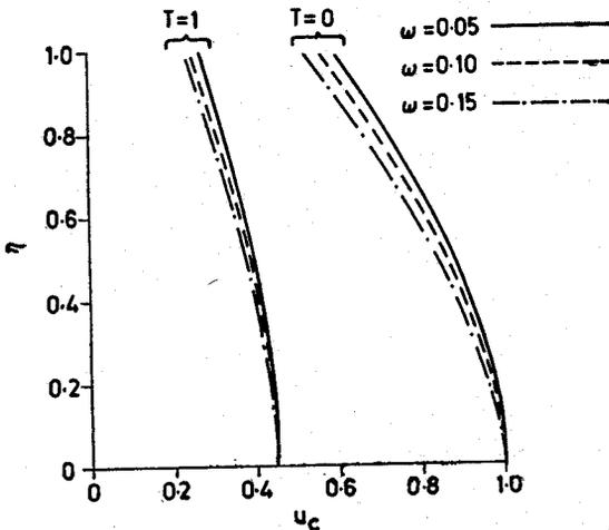
Figure 5. Velocity distributions of the clean gas along with the direction of motion of the plate.
