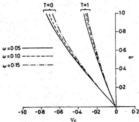
Figure 6. Velocity distributions of the clean gas in a direction normal to the direction of motion of the plate.
