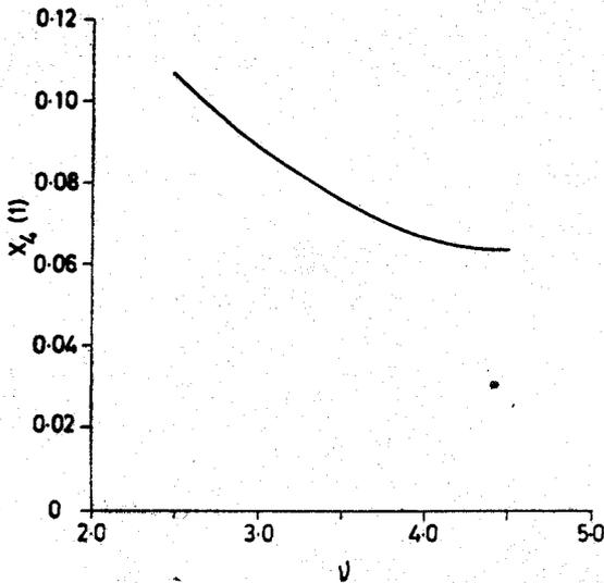
Figure 6. Ballistic Factor  $X_4(1)$  vs.  $v$ .
