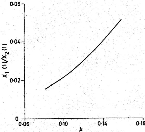
Figure 3. Ballistic factor  $X_1(1)/X_2(1)$  vs.  $\mu \left( = \frac{S}{2\pi l^2} \right)$ .
