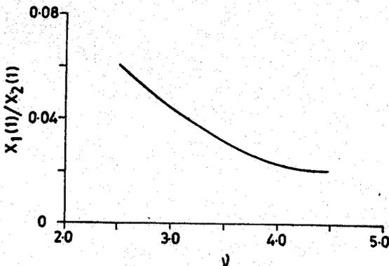
Figure 5. Ballistic factor  $X_1(1)/X_2(1)$  vs.  $\nu \left( = \frac{2S}{\pi d^2} \right)$ .
