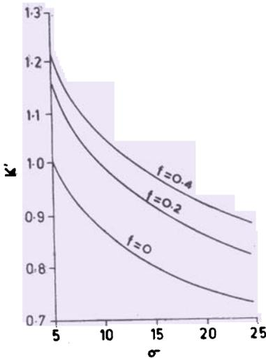
Figure 4. Variation of  $k'$  against frequency  $\sigma$  for different values of mass concentration of dust  $f$  (Eqn. 41).
