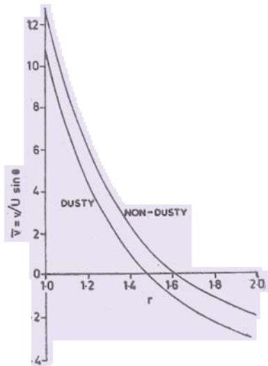
Figure 2. Variation of  $\bar{v} = v/U \sin \theta$  across the annular spaces between two concentric spheres  $r = a, r = b$ .
