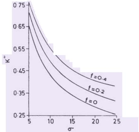
Figure 5. Variation of  $k''$  against frequency  $\sigma$  for different values of mass concentration of dust  $f$  (Eqn. 42).
