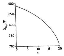
Figure 3. Variation of drag ratio Da, t/D of dusty fluid drag to the clean fluid drag on sphere r = a.
