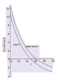
Figure 2. Variation of  $\overline{v} = v/U \sin \theta$  across the annular spaces between two concentric spheres r = a, r = b.
