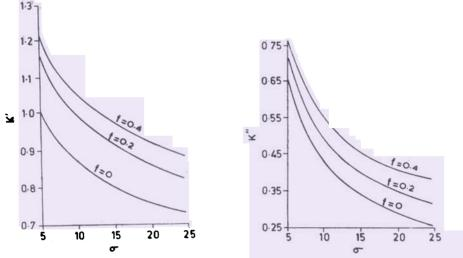
Figure 4. Variation of k' against frequency  $\sigma$  for different values of mass concentration of dust f (Eqn. 41).
