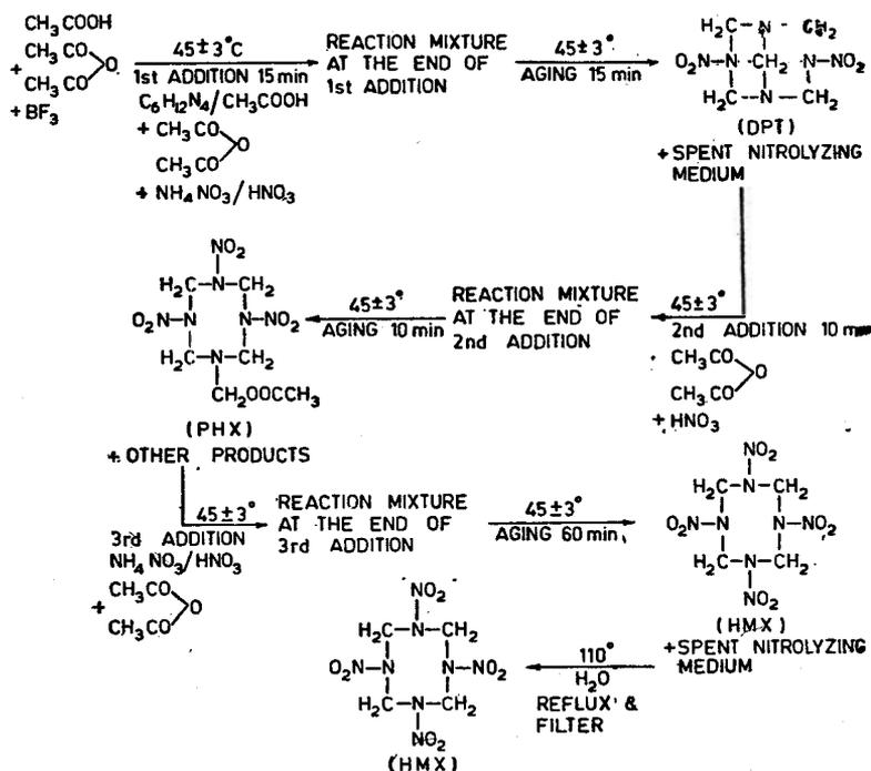
Figure 1. Flow diagram for the nitrolysis of hexamine.
