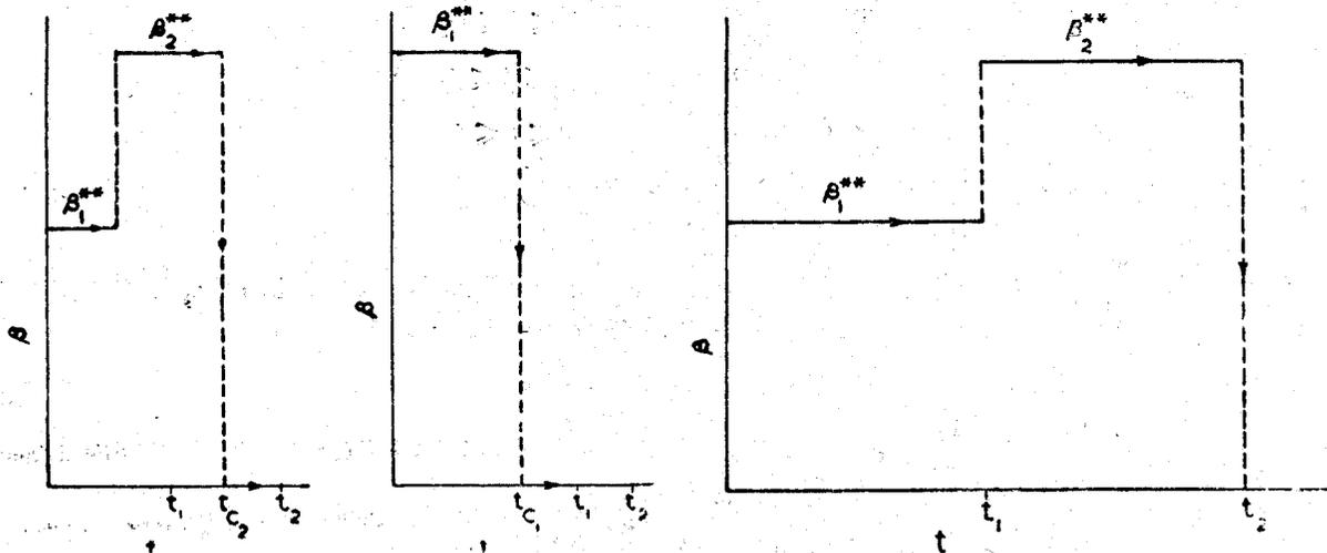
Fig. 1—Mass flow rate versus time for a two-stage rocket for achieving maximum height.
